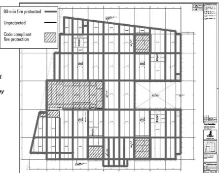
Figure 1: Floor arrangement at Ropemaker Place in London. Beams highlighted in thick grey are fire protected; beams not highlighted are unprotected. This solution represents the state of the art capability in structural fire engineering.
